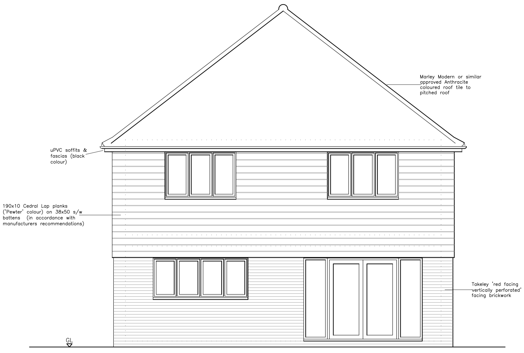
rear elevation scale 1:50
