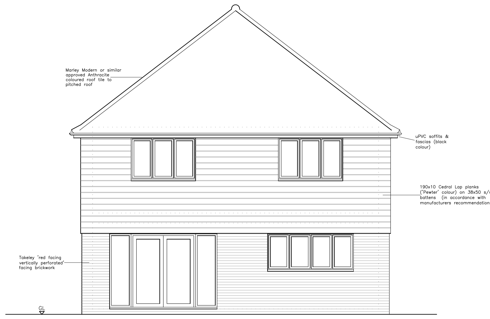
rear elevation scale 1:50
